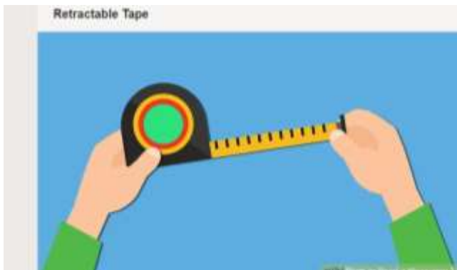
Fig 13 Catch the hooked end on one side
